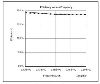
Figure 15. Efficiency vs. frequency
